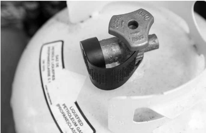
the pressure for which it was designed, eventually resulting in a crack or fissure in the container, thus introducing normal atmospheric pressure to the liquefied gas which causes it to flash to vapour. The vaporizing liquid will increase the pressure in the container until the container explodes. In addition to flying container fragments,
